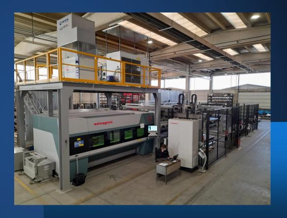
Automated sheet load/unload functions with storage tower system Unattended operation and automatic sorting devices
