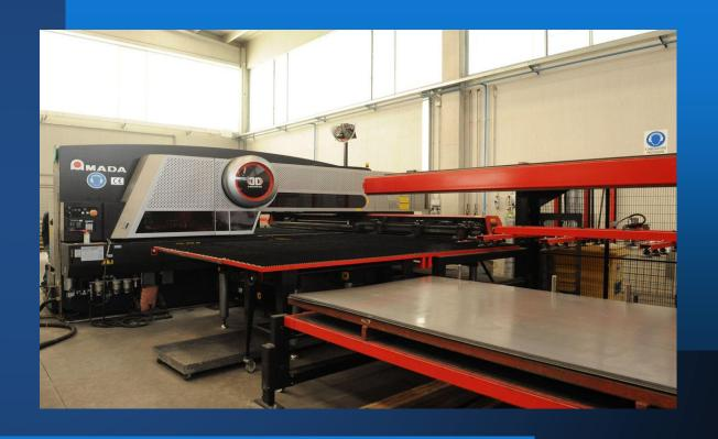
Possibility to carry out countersinks, small deformations (winglets, air shafts) Possibility to deform from below. Automatic loading/unloading devices
