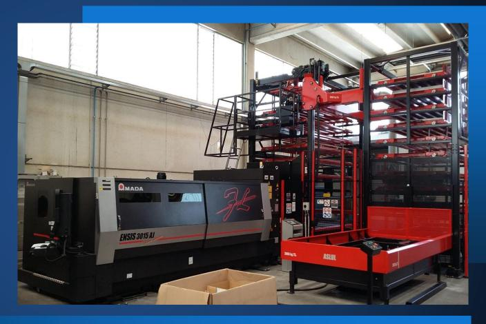
Automated sheet load/unload functions with storage tower system Unattended operation
